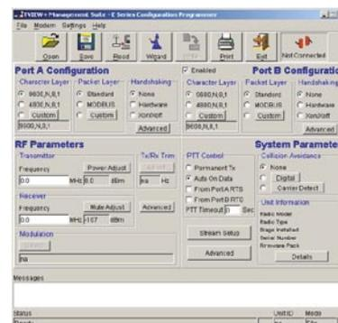
Click on the "Read" button. This will read the configuration of the radio. The "connection" symbol in the top right hand corner of the screen will turn from **Red** to **Green** to indicate a successful configuration connection.
