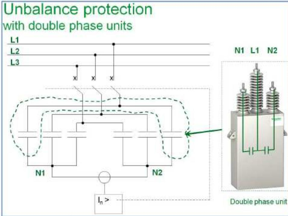
This is the single line diagram of a double star connected bank using 3 Double-phase capacitor units.
