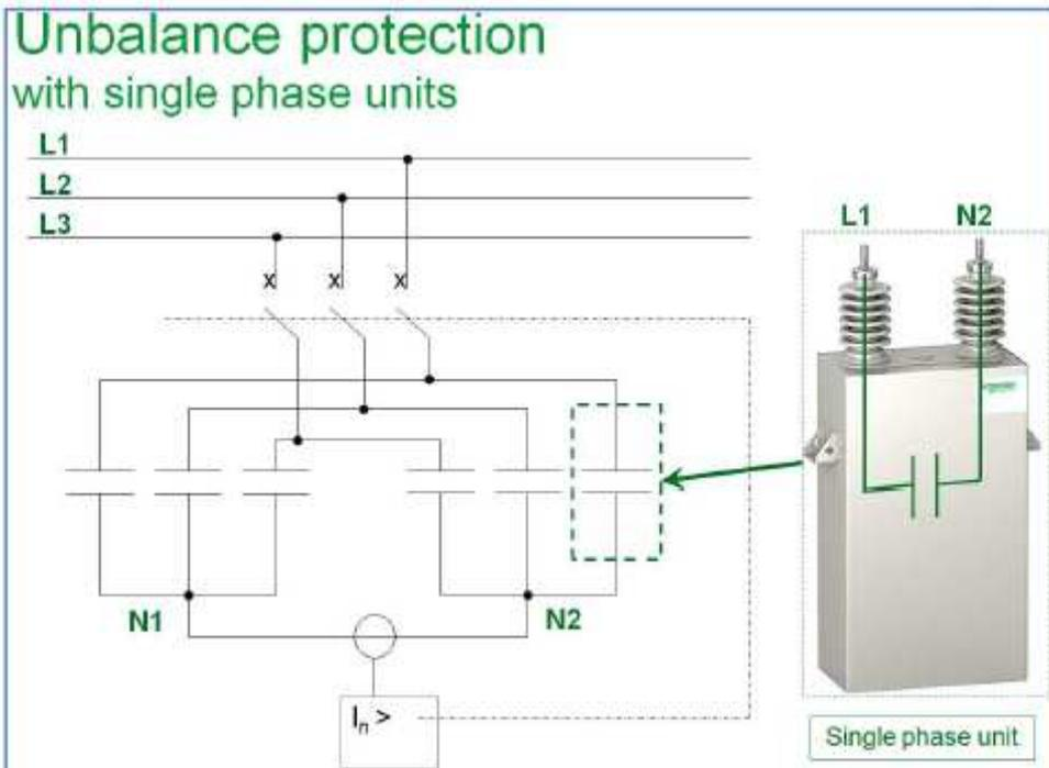
This is the single line diagram of a double star connected bank using 6 Single-phase capacitor units.
