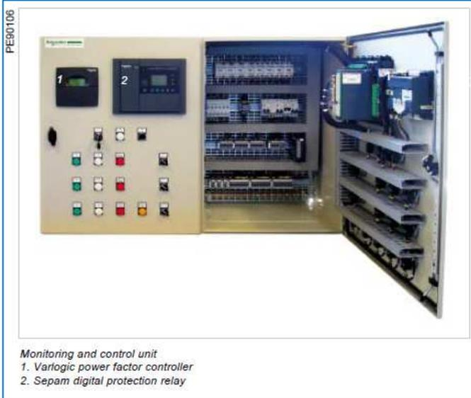
For indoor type capacitor banks: the control and protection devices can be “Door mounted” for IP21 capacitor bank. Otherwise it shall be inside a LV compartment of the capacitor bank” (IP23 to IP54) or in a separate “Control Box”.
