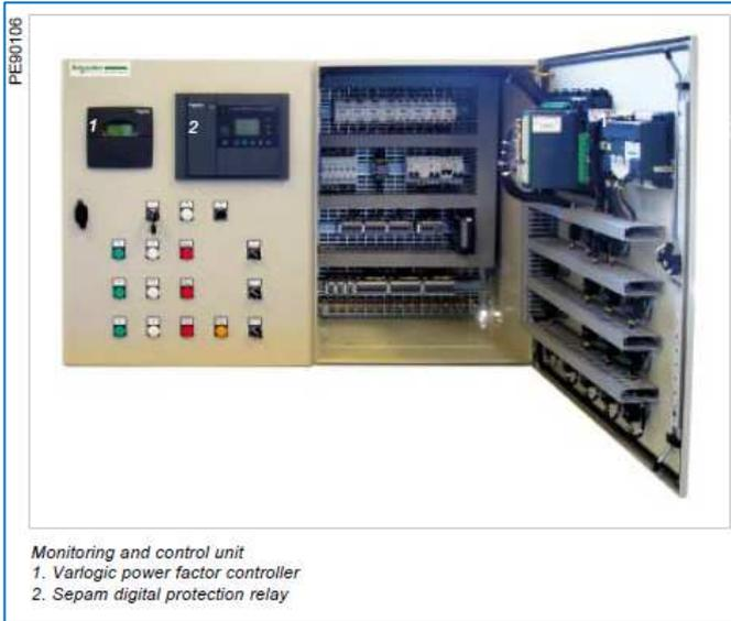
For indoor type capacitor banks: the control and protection devices can be “Door mounted” for IP21 capacitor bank. Otherwise it shall be inside a LV compartment of the capacitor bank” (IP23 to IP55) or in a separate “Control Box”.
